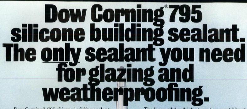
Dow Corning® 795 silicone building sealant. Our one-component, low-modulus, architectural-grade sealant. It has excellent adhesion, without any primer, on glass, metal, masonry, plastic, and just about any other building material you can name.
