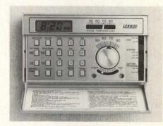
An electronic thermostat, Model T 800 for homes, is programmable to regulate both heating and cooling cycles for a period of five or seven days. According to the manufacturer, it can replace an existing single-stage thermostat without additional wiring. Temperature settings can be varied throughout the day to meet occupants' needs and conserve energy. Liquid crystal digital display shows time. Lennox Industries, Inc.
