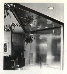
Designer Series ceiling panels of antique glass, in a 2' x 2' size, rest on an exposed grid. The tegular edges of panels extend below the grid, making the grid slightly recessed from the ceiling surface. Panels have a sound absorbence value of NRC-.60 and offer easy access to the plenum. Armstrong Cork Company.
