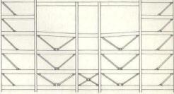
1969: UNBUILT BRACED FRAME DESIGN, NOTE ECCENTRIC BAYS
