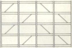
1971: FIRST ECCENTRIC BRACED DESIGN (UNBUILT)
