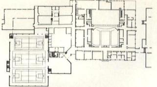
Designing for tornado or earthquake resistance usually has ramifications in the plan organization and detailing of a building. Architects Marshall & Brown of Kansas City designed the Chillicothe High School with adequate refuge from tornado in mind. Below Dr. Irving Oppenheim has invented a spring-embedded door frame design which can accommodate movement in the wall plane while maintaining an operable door for emergency use.
