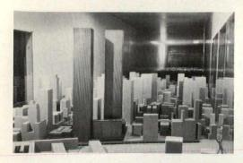
(Above) Systematic methodology for tall building wind analysis began with wind tunnel testing for the World Trade Center. (Center) Aerolastic models are constructed to simulate dynamic response to wind loading. (Right) Boston's Federal Reserve Bank is also modeled in rigid form for exterior pressure analysis. (Below) Similar model techniques are used for low-rise structures. Simplified loading blocks also improve the effectiveness of the designed wind response of the structure.
