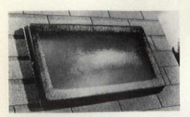
The Tri-Therm Skylight has an outer dome of GE's Protect-A-Glaze® sheet and an inner diffuser panel of GE's Lexan® structural sheet which combine to provide three layers for high impact strength and superior thermal properties. The outer dome has a pebble finish and comes either clear or tinted for solar control. The skylights provide daylighting and thermal gain to help reduce energy requirements. They are lightweight, economical, and easy to install. Faulkner Plastics.
