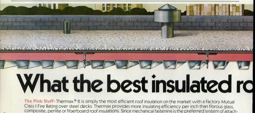
ment to steel decks, use Insulfast rapid fastening nail/disc system – a pneumatic gun and oxide-coated nails for
