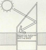
SKYSHAFT INSULATING AIR CHAMBERS
