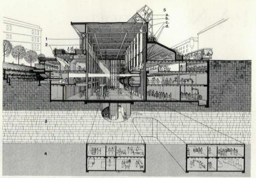
Trombe wall. 2 Solar shading. 3 Earth sheltering.
