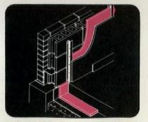
Exclusive! Z-Furring System for insulating masonry and concrete walls.
