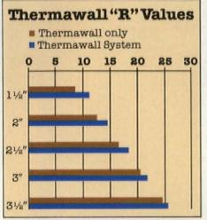
Note: Thickness includes 1/2" gypsum. Aged "R' values tested at 75° mean temperature
