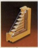
Slimshade<sup>®</sup>, set between the panels of the Double Glass Insulation System, cuts heat loss and solar heat gain. (U value, .39; R value, 2.56; shading coef-ficient, .34)\*
