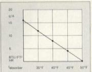
q/A = Heat which must be transferred to the exposed surface by blood circulation in order to maintain a "comfortable" 50°F skin temperature while radiating to a cool absorbing surface at temperature t
