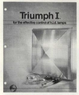
Triumph I prismatic control lens for 2' x 2' HID light fixtures is described in a 12-page, full-color catalog. The lens distributes lighting 40-45 degrees from
