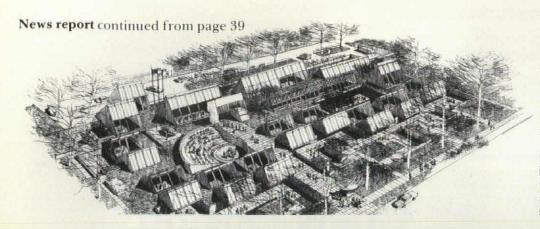
bring light into classrooms and circulation spaces immediately below them; solar collectors are mounted above storage and mechanical spaces.
