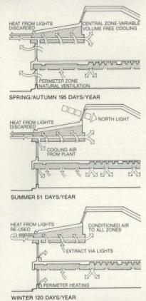
Hereford and Worcester County Hall: As shown in the diagrams above, the building was designed with heat recovery in mind for the appropriate season. Over 18,000 sq m of space provides a working environment for 710 people. A high thermal mass, double glazing, automated lighting controls, and air-handling light fittings all contribute to the energy efficient design. Architects: Robert Matthew, Johnson-Marshall and Partners.
