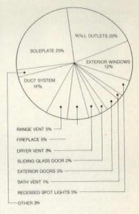
This chart shows the relative contribution of infiltration sources in a typical residence. (From Electrical World, Nov. 1, 1978.)
