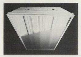
A three-lamp fluorescent troffer, designed with one less lamp for energy saving, can further cut energy costs because it is wired for one, two, or three lamp operation. The troffer is  $3\frac{1}{2}$  in. deep, has a door that can be hinged
