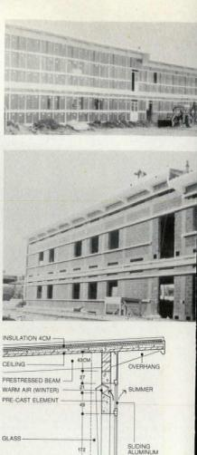
GLASS AIR LAYER SOLID CONCRETE BLOCK PAINTED FRESH AIR
