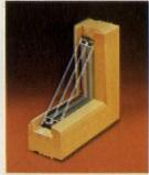
Triple Insulating Glass, ideal for large fixed units and sliding glass doors, provides outstanding energy conservation. (U val-ue, .35; R value, 2.86; shading coefficient, .74)\*\*
