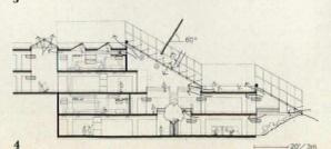
Natural draw (above) brings site through complex. The solar court sections (left) indicate 1) passive solar heating, winter; 2) passive night sky radiation/diurnal cooling, summer; 3) passive heating, night; and 4) day natural ventilation cycles.
