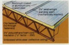
solar heat. Inside, the galvanized steel facing is factory-painted to provide a highly reflective (65%) ceiling.
