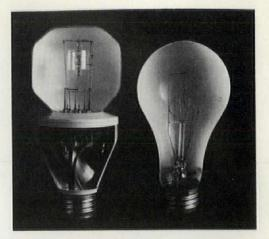
The 'Electronic Halarc' bulb is an energy-saving bulb that fits standard household fixtures. To become available in 1981, the bulb has electronic controls in the base and an arc tube in the top. It has high and low settings, with the high setting producing as much light as the 150-watt setting of the typical three-way bulb using about one-third the energy. General Electric, Lighting Business Group. Circle 118 on reader service card
