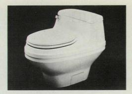
The Series 4000 water closet, a one-piece, low-silhouette, water-saving fixture, is made from a strong, durable honeycomb material blended of polyvinyl chloride, polypropylene, and urethane foam. The unit weighs only 29 lb, yet it can withstand a static load of 3000 lb. Cost is approximately half that of most one-piece china units. Colors are white, bone, and parchment. Delta Faucet Co.
