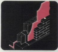
Masonry Cavity Wall Insulating System.
