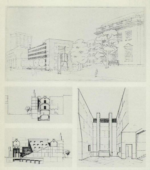
The Fogg Museum addition (top), with the present Fogg at right, Gund Hall at left, and William James Hall behind. Left, top: section showing street-side offices and three gallery levels (shaded) flanking main stairway. Left, bottom: section through main stairway. Above, right: entrance hall.
