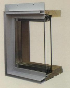
Super energy-efficient quad glazing is offered in direct set units only. Quad pane units are 1<sup>3</sup>/<sub>4</sub><sup>"</sup> thick, consisting of two lites of film suspended between the outer layers of glass. The units rate high on solar transmission while insulating better than triple pane units.
