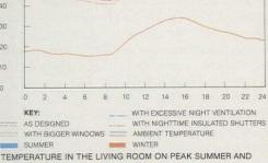
The analysis shows that without air conditioning the house will overheat in the summer. Actual temperatures will probably be somewhat lower because of the lower altitude (1000 ft) of the source used for weather information in the analysis. Nighttime ventilation during summer months substantially reduces peak temperatures.
