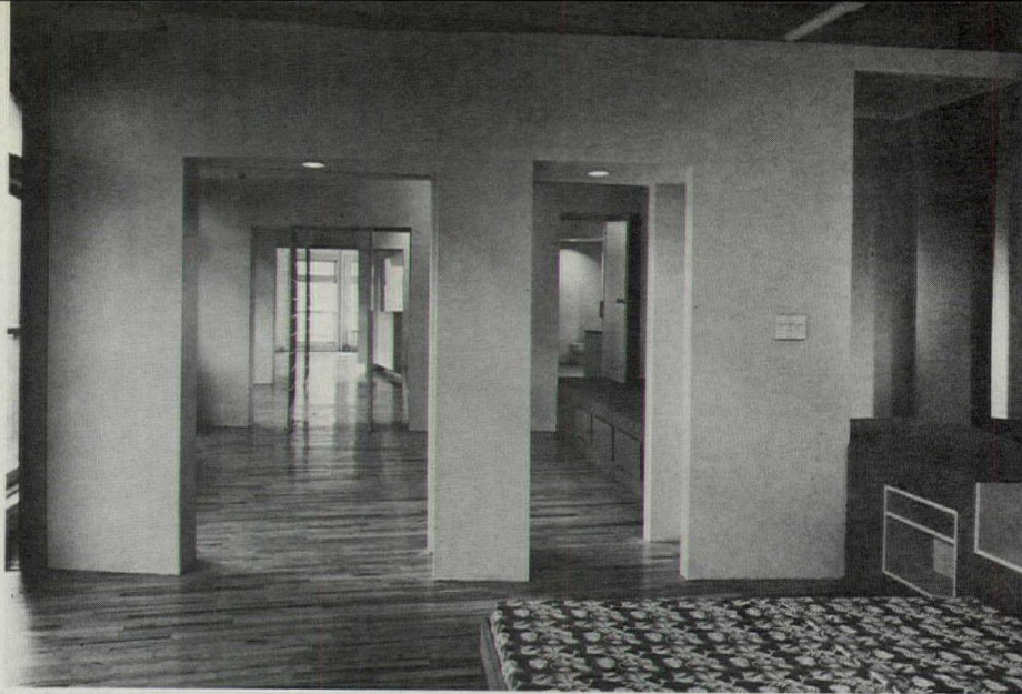
Double partitions of airfoil shape in plan divide loft along lines of original bays (above). Kitchen (left) occupies angular form projecting into living space; raised floor extends through bath and forms platform along storage wall in bedroom.
