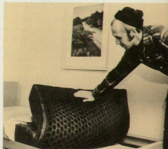
Neoprene foam mattress, installed for comfort and durability, is still comfortable after 21 years of service on oil tankers.
