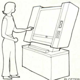
STEP 6 PLOTTER PRODUCES ANY LAYER OR COMBINATION OF LAYERS IN FINAL WORKING DRAWING QUALITY ON DEMAND. 3-5 DAYS
