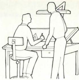
STEP 3 DESIGNER AND DRAFTSMAN COORDINATE CONSULTANTS' DRAWINGS AND REDRAW STRUCTURAL AND MECHANICAL ELEMENTS ONTO ORIGINALS. 2-4 WEEKS
