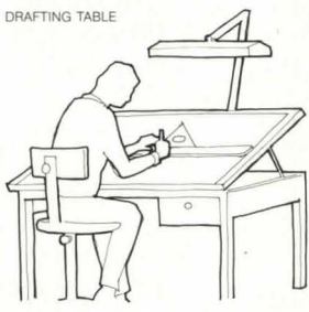
STEP 6 UPON RECEIPT OF DRAWING DESIGN CHANGES, DRAFTSMAN MAKES CORRECTIONS ON CLEAR FILM OVERLAYS IN INK. 3-5 WEEKS
