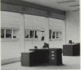
MIT's Rectilinear Sky Simulator; inside there is a luminous ceiling surrounded by vertical mirrors that simulate the overcast sky (far left). Model being tested in the simulator
