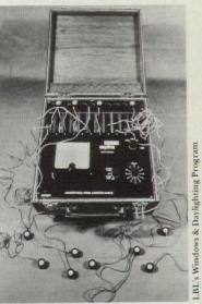
Megatron Architectural Photometer, one of the more sophisticated measurement devices now being made (must be ordered from Britain), was specifically designed for daylighting analysis.
