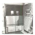
SCP 5: A Solid Core Door 3/4" thick. Standard door has Anodized Aluminum, Top Panels, 18 gauge steel center panels (SS front, Galv. rear), 14 gauge high carbon steel kick plates. Optional decortop panel, rub strips & jamb guards shown. Applications same as "LWP 3"
