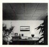
Fabrique<sup>TB</sup> ceiling panels are molded of 1-inch or 11/2-inchthick fiberglass in standard 2' x 2'or custom 5' x 5' size. They have a Class A fire-hazard rating and a sound-control rating of NRC .90 or 1.00 and NIC' of 18 or 20. The panels can be covered with a choice of fabric colors and weaves or COM, Donn Corp. Circle 116 on reader service card
