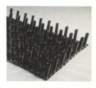
Hydraway™ drain to keep water from entering building foundations or basements consists of heavy-duty filter fabric permanently bonded to an internal supporting core. Water passes through the filter fabric, then flows into the core conduit around the perimeter of the foundation, and empties into a drain outlet such as a storm sewer. The system is fastened directly to the foundation with a nail gun or glued to the wall with mastic. Monsanto Company. Circle 215 on reader service card
