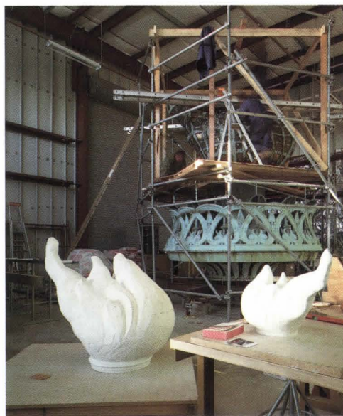
The statue's flame (top) was originally all copper-clad and gold-leafed; the glass was added later with the installation of interior lighting. The replacement flame (above), seen in model form, will return to the original design, with high-intensity lights, hidden behind the torch's railing, shining on the nonspecular gold finish. A University of Denver team used photogrammetry to record the old flame.
