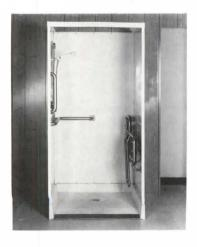
Shower Model 99H for the handicapped has a seven-inchhigh terrazzo base with stainless steel ramp. Threshold height is one-half inch for wheelchair access. It has a pressure-balanced single-lever mixing valve, wall-hung and hand-held shower, wraparound horizontal grab bar, vertical straight bar, and folding transfer seat. The unit is constructed of galvanized bonderized steel walls with one-piece top frame and integral curtain rod. Fiat Products, Inc.
