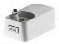
An extended wall-mounted drinking fountain, Model 1075, is a wheelchair-accessible unit. Constructed of white or tan polymarble with rounded corners for a smooth appearance, it is equipped with polished chromium-plated vandal-resistant bubbler and front push plate. It also has a vandal-resistant bottom plate and integral mounting brackets. Haws Drinking Faucet Co.
