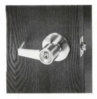
The 8K lever handle lock, which meets handicap codes, is designed with all the functions of a keyed cylindrical lock. It has a breakaway knob driver, to resist forced entry, that can be adapted to existing 8K cylindrical locks. The hand of the lockset can be changed quickly to either right or left without removing keyed knob. Best Lock Corp.
