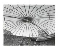
Rolladome is a motor-driven operable dome skylight of galvanized steel with bronze acrylic glazing. Opening the skylight vents heat buildup in summer, and single glazing allows maximum solar gain in winter. Rollamatic Roofs, Inc. Circle 120 on reader service card
