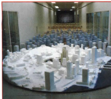
4 Model of Hong Kong in wind tunnel
