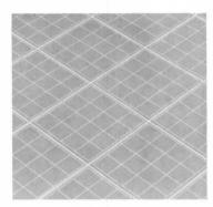
Geometric Italian ceramic floor tile is produced by the monocuttura method, a single-fired process that results in a denser surface and stronger, longer lasting glaze bonding. The 8" x 8" frostproof, flat-back tiles are 3/s-inch thick, in white, gray, bone, and sand, and are suitable for residential and commercial applications. Ballack Corporation.
