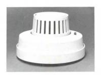
PEC-3 photoelectric smoke detector for commercial, industrial, institutional, and residential applications has a field cleanable photo chamber. The UL-approved unit has an optional concealed locking mechanism to prevent unauthorized removal of the detector. It can be intermixed on the same zone circuit with other Pyrotronics low-voltage detectors. Pyro-
