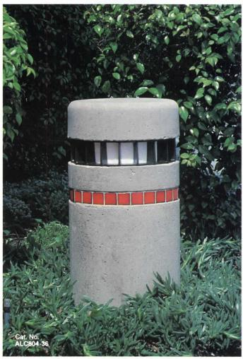
**Durable Lighting constructed** of precast concrete, reinforced with steel rebar, providing vandal and corrosion resistances for a long time. A cast aluminum grill with an inner high impact acrylic diffuser encloses a variety of energy efficient H.I.D. lamps. Choose from (3) sizes in a textured or smooth concrete finish. Concrete colors and ceramic tiles are available.
