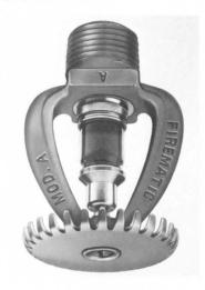
Fire-Master bulb sprinklers feature tapered ½-inch orifices that ensure uniform spray distribution for maximum fire protection without turbulence. They come upright or as pendents with orange, red, yellow, or green bulbs. Sprinklers are rated at 135 F, 155 F, 175 F, and 200 F, and are UL listed and Factory Mutual approved. Finishes are bronze or polished chrome. Firematic Sprinkler Devices. Circle 104 on reader service card
