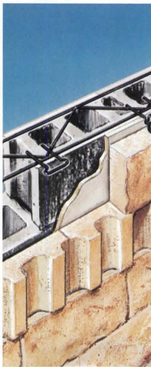
An insulated concrete masonry cavity wall under construction.
