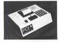
Prime-Color: Illumination quality meter is a sophisticated, handheld, computer-operated lightmeasuring device. Circle 232 on reader service card
