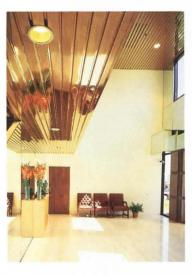
Apollo linear metal ceiling panels are one inch in depth, with rounded corners. Strength of the deeper panel allows longer spans with fewer splices. Splices are formed, rather than rolled, resulting in straighter, flatter joints. Panels are made of aluminum and steel in a wide range of colors and finishes. AEP Span.
