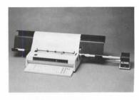
The Open End Typewriter uses memory printing units, particularly the IBM Wheelwriters® and Quietwriters®. Features include 31K memory, editing capabilities, automatic functions, lift-off correction, many type styles, and ease and speed of operation. All functions are controlled from the regular keyboard. The print is letter quality. Diagram Corporation.
