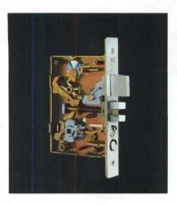
30H Series locksets offer improved security. A patented roller bearing knob mechanism (arrow) allows improved knob action through lower and consistent torque value. The case is heavy gauge steel, and solid machined cylinder rings are tension spring mounted. Knob hubs and locking mechanisms are heavy steel. Optional high security cylinder on 36H/37H series complies with ANSI 156.13. Best Lock Corporation.
