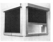
Lite-Tite shades are vinyl-coated fiberglass housed in extruded, anodized aluminum frames and attached to a roller mechanism at the top of the frame. They are completely lightproof, providing protection in light-safe environments such as photo labs, laser surgery centers, heat catherization labs, art galleries, and computer rooms, where both light control and heat control are important. The shades are easily cleaned and sanitized. They are offered in a variety of colors. O.C. Steele Co.
