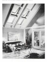
Sunrise venting and fixed roof windows use Low-E insulated, tempered glass with softcoat glazing. The transparent coating eliminates 71 percent of UV rays. There are nine models, each with inside screens attached and hardware baseplate installed. Roto Frank of America,
