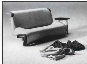
**Luck Sofa**, by Japanese designer Toshiyuki Kita, is constructed of a welded steel armature encapsulated in expanded polyurethane foam. It is padded with Dacron fiberfill and then upholstered. The legs are molded self-skin black urethane foam capped with nylon glides. Optional removable covers stretch over the body. AI.
