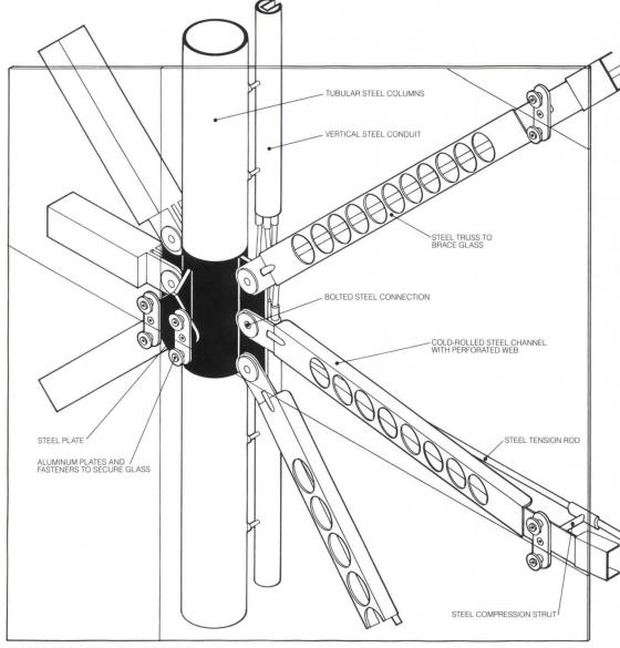
AXONOMETRIC VIEW OF COLUMN AND TRUSSES
