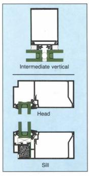
United States Aluminum Corporation is now offering the Series SG 450 Structural Silicone Glazing Ribbon system engineered for low and high rise glazing projects.
