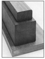
Pau Lope is an especially dense and rot-resistant wood imported from Brazil. Its resistance to splitting, splintering, and warping makes it useful in outdoor applications, as does its 60-year life expectancy. Greenheart Associates, Inc.
