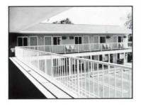
**Pipe picket railings Series 550** of nonwelded aluminum are strong, durable, and require no paint maintenance. Fittings are aluminum extrusions and castings. Railings are made to customer specifications in lengths up to 24 feet and heights of 30, 36, 42, and 48 inches. Finishes are white, bronze, dark bronze, brown, and black baked-on enamel or satin and Duranodic anodized. Superior Aluminum Products.
