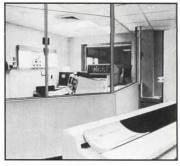
Lead-Plastic x-ray room shielding, Clear-Pb®, combines light transmission with radiation shielding. Prefabricated modular barriers and windows are used in x-ray and special procedures rooms. Clear-Pb is available in 0.3 to 1.5 mm lead equivalencies and sizes up to 6' x 8'. Nuclear Associates.
