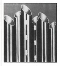
Colored stainless steel pipes are a solution to identification problems. Colors range from black through bronze, green, blue, red, gold, and champagne. The color is part of the material, created by application of a thin film of chrome oxide. Prismatic Div., B&M Finishers.
