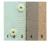
Senerthik high impact-resistant exterior insulation and finish system. (1) AMOFOAM, (2) mechanical fastener, (3) reinforcing fabric, (4) ½" polymer modified base coat, (5) protective finish coat
