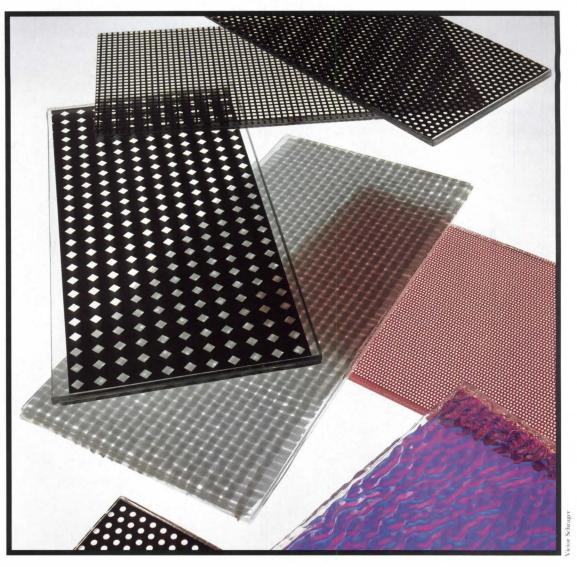
light whose angle varied with the desired angle of the louvers, and then heating the glass in a kiln. The notion was that the angle prescribed for the louvers would vary according to the glazing's position and height in the building and thus provide shade from the sun without restricting views from the windows. But, in an eleventh-hour decision by the client, another, more conventional, glass was chosen for use in the building.
