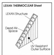
LEXAN polycarbonate sheet is an impact-resistant glazing for skylights and high-traffic or bullet-resistant applications. For thermal protection and high-impact strength, a double-walled, extruded LEXAN Themoclear sheet is available. General Electric Company.
