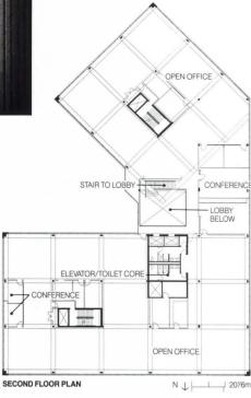
feeling depends somewhat on the ceiling height. Floors with ten-foot heights look less like mazes than floors with the more typical ceiling height of 8'6". If raised floors are used to accommodate power needs, floor-to-floor heights must be even higher.
