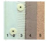
Senerthik high impact-resistant exterior insulation and finish system. (1) AMOFOAM, (2) mechanical fastener, (3) reinforcing fabric, (4) 1/4" polymer modified base coat, (5) protective finish coat.
