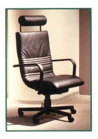
Physio-Class Seating employs a chair shell of semi-rigid molded plastic that flexes with upper body movement. Without special controls, it provides support through normal postural changes. The chairs can be fixed to accommodate those who work at screens or in other capacities where the body leans forward. The chair's tilt control is designed to keep the user's feet on the floor during movement, thus reducing stress on legs and knees. VOKO U.S., Inc.
