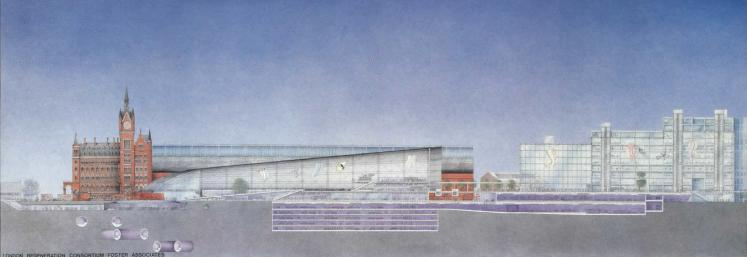
Section through vaulted space showing connection through new office buildings to oval park (far right).
