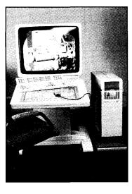
A technical workstation called InterPro 3070 incorporates a central processing unit and new 27-inch display that doubles the area with the same resolution as a 19-inch screen. Intergraph. Circle 115 on reader service card
