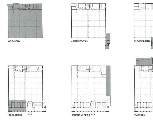
The assembly of a post office (above) combines elements that are sized and selected according to local needs.
