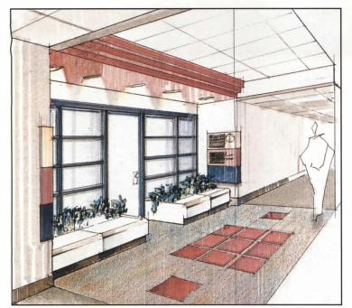
Figure 1. Destination design includes recessed entry niche, enhanced lighting, carpet inset, built-in planters, tiered soffit, and glass.
