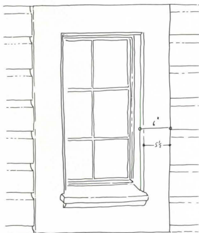
Examples of the meticulous, yet sketched, detailing Krier provided include the finely-crafted windows, sills, and surrounds (above and below, left), the various column capitals (below right, above center and right, and facing page), and the roof brackets.
