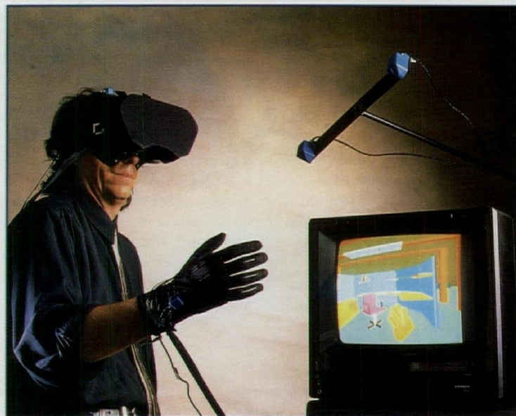
Autodesk's Cyberspace, with the aid of sensors in gloves, goggles, and microphones, enables our physical interaction with computer-generated "virtual reality".
