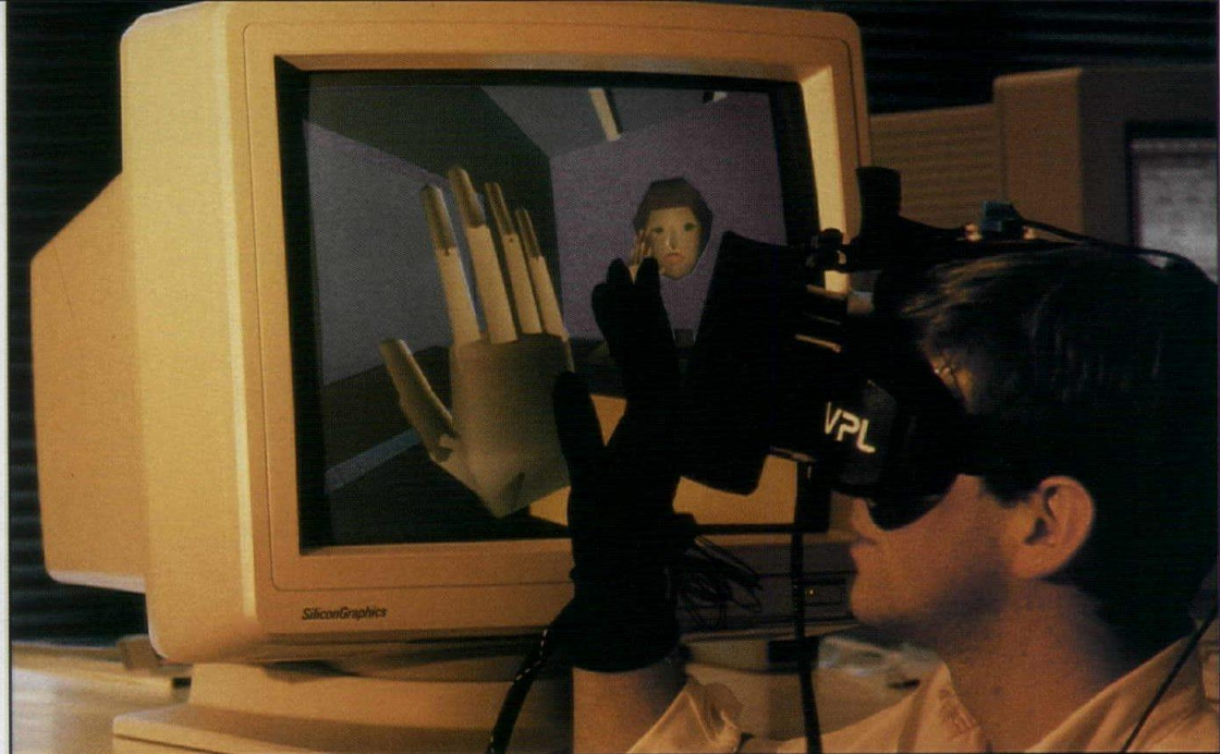
VPL Systems provides complete virtual environment systems including workstations, "Datagloves," and "EyePhones," which can convert hand gestures and head movement into electronic signals.
