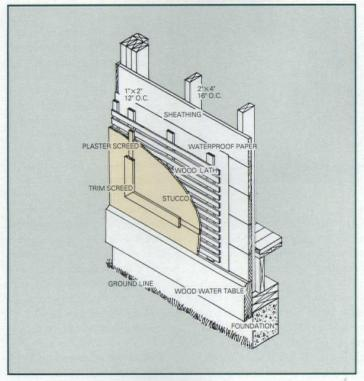
CUTAWAY AXONOMETRIC OF A WOOD-FRAMED STUCCO WALL
