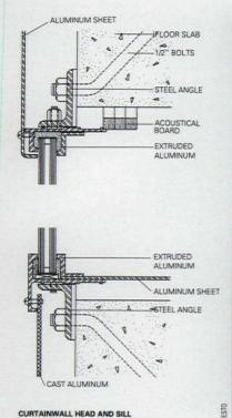
The Equitable Building in Portland, Oregon, designed by Pietro Belluschi in 1948, is an early example of an aluminum curtain wall. The wall is connected and anchored to the structural reinforced frame with carbon steel angles. The curtain wall is made up of extruded aluminum profiles, cast aluminum panels, and sheet aluminum covers.
