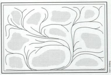
1 Diagram of splits in the roofing membrane.
