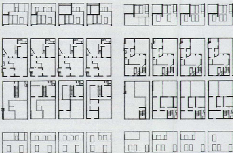
VARIOUS HOUSING UNITS, (FROM TOP TO BOTTOM) SECTIONS, FIRST FLOORS, SECOND FLOORS, AND ELEVATIONS
