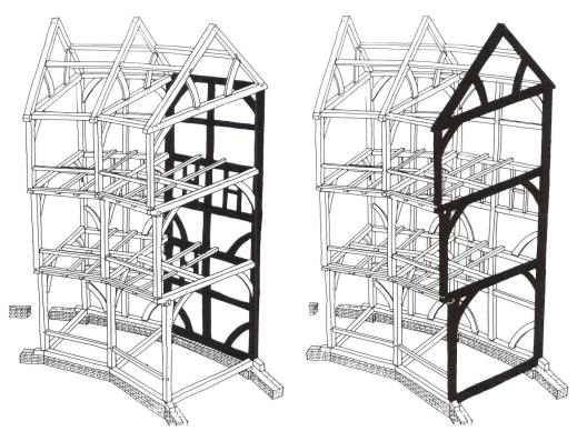
DIAGRAMS OF TIMBER BAYS (BLACKENED PORTIONS SHOW HOW THE THREE-DIMENSIONAL STRUCTURE CAN BE RATIONALIZED INTO TWO-DIMENSIONAL ELEMENTS THAT CAN BE FABRICATED LYING FLAT IN THE CARPENTER'S BUILDING YARD)
