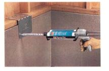
This low-cost epoxy system for retrofits in concrete or masonry provides stronger anchoring than can be achieved with mechanical anchors. Epoxy-Tie™ bonds with surrounding concrete; the anchor is less prone to sideburst during close-interval installation. The system has a higher resistance to moisture and vibration than mechanical anchors. **Simpson Strong-Tie® Company, Inc. Circle No. 367**
