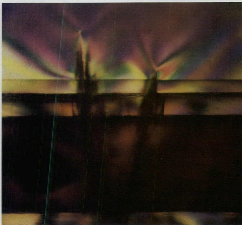
MICROSCOPE PHOTO OF POLYMER-COATED GLASS PIPETTE WITH ADHESIVE BEING RELEASED
