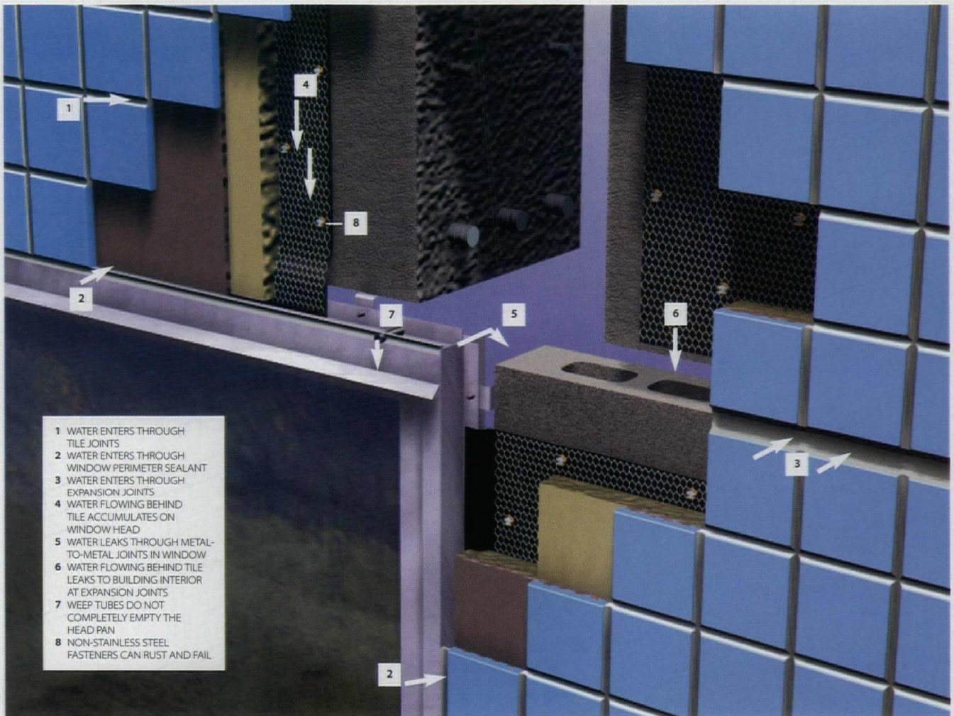
1 CRITICAL POINTS IN DETAILING TILE CLADDING
