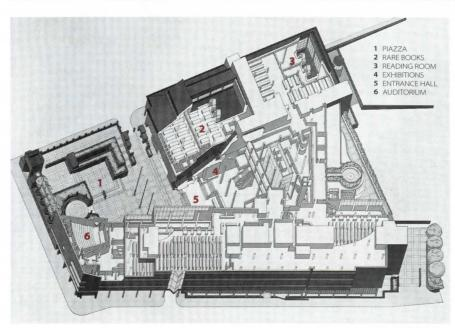
The new British Library by Colin St. John Wilson has a piazza on top of four levels of underground stacks. The axonometric shows its organization.
