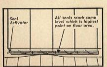
"T" FLOOR SEAL ON TORJESEN FOLDING PARTITIONS Effects 100% Closure Regardless of Floor Contour!
