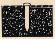
Steel to concrete, such as conduit and pipe clips; duct straps, angles, brackets and braces.
