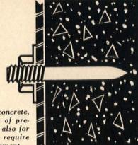
Threaded studs to concrete, such as attachment of predrilled materials — also for materials that may require removal or replacement.
