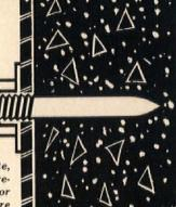
Threaded studs to concrete, such as attachment of predrilled materials — also for materials that may require removal or replacement.
