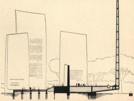
Section shows tallest shaft cantilevered from monolithically poured slab.
