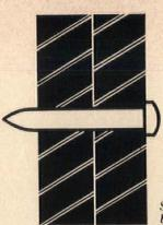
Steel to steel, such as angles and brackets to beams.
