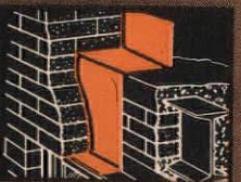
Spandrel beam waterproofing
