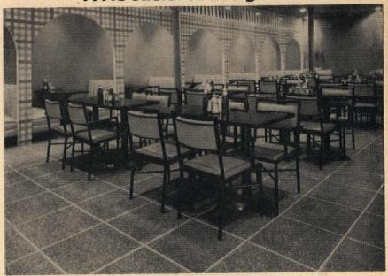
TERRAFINO is the original 12"x12"x3/16" flexible tile with real #1 and #2 marble chips permanently bedded in a tough epoxy plastic matrix. The TERRAFINO floor pictured above (Calico Kitchen Restaurant, Cheltenham, Pa.) is a typical example of the benefits to be derived from this modern way to install terrazzo.
