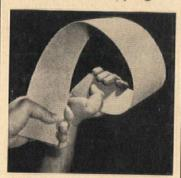
Silicone rubber material vulcanizes to a flexible concretelike substance. It is water-resistant, and, with a primer, may be used as a protective coating over concrete, steel, or wood. "Silicone Traffic Topping" is recommended to be trowelled onto horizontal surfaces, and may also be used as a grout for tile and stone, or to repair cracks. It is available in fade-resistant colors. General Electric, Silicone Products Dept., Waterford, N. Y.
