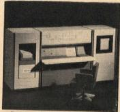
System 10, least automated of the four, controls up to 100 systems. It can tell actual temperature set points and damper positions, and operator can make adjustments. A solid-state scanner alerts operator to off-normal conditions with an audible alarm and then prints out information. A multichannel recorder can automatically record temperatures for making system analyses or to observe trends.
