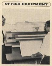
Combination developer and printer for reproducing drawings has added the ammonia system to the developer section. Ammonia control container needs no venting and, after being filled, the "Diazo-Jet" may be left on all day with no further attention. Care and operation of the
