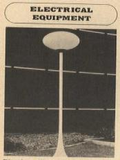
Plastic ellipsoid luminaire atop a cast-aluminum pole for outdoor lighting accommodates up to 400-w mercury vapor or 500-w incandescent light. Pole (8', 10', 12', or 14' high) is finished in baked acrylic - white, black, or dark bronze. Luminaire, 34" dia., has built-in reflector. Suitable for parks, campuses, parking lots, street lighting, etc. Kim Lighting, 1467 N. Lidcombe, El Monte, Calif. 91733. Circle 110, Readers' Service Card
