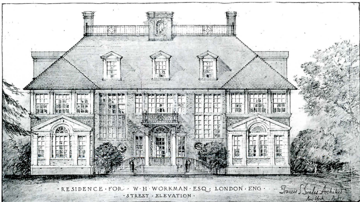
Figure 23. A scale study of an elevation on tracing paper, rendered in lead pencil, for discussion with client. Residence for W. H. Workman, Esq., London, England, Francis S. Swales, Architect
