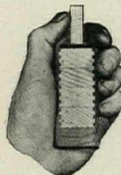
Cross-sectional sample of COM- POUND construction, showing 3/16 inch sawn veneer tongue-and- grooved to core.
