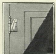
Half-surface and fullsurface butts are easily applied and presentaneatfinished appearance.
