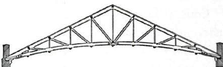
Howe Trusses with Straight or Curved Lower Chords
