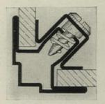
Sash B-1 and Corner Bar B-2 of "B" construction (Full Size). Sufficiently sturdy and graceful for the largest and finest store fronts.
