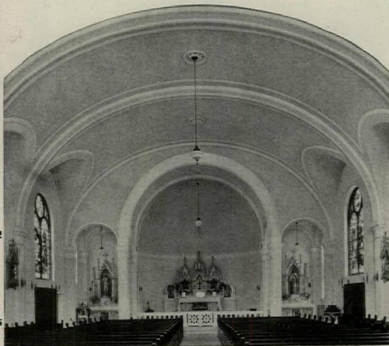
Illustrating sharpness of detail in design and absence of cracks--typical of lime plaster. Holy Trinity Church, Kansas City, Mo. Brinkman and Hagen, Architects, Emporia, Kans. W. F. Gosche, Contractor. Harry Walters, Plastering Contractor, Kansas City, Mo.
