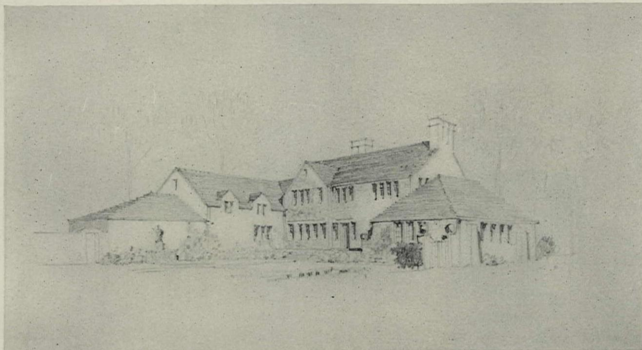
FREEHAND PERSPECTIVE SKETCH MADE WITHOUT PLAN OR VANISHING POINTS
