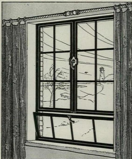
Minimum fresh air ventilation without drafts, for cold or stormy weather.
